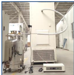
LN 2 /CO 2 backup system
